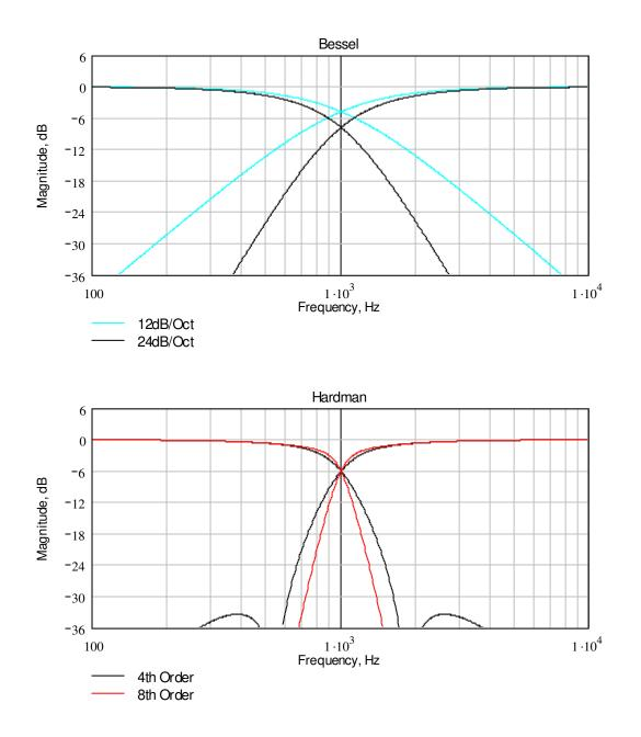
The following plots show the magnitude response (frequency response) characteristics of the various equalization filters available within the DNA 5K4c amplifier. These are all shown at a frequency of 1kHz.
