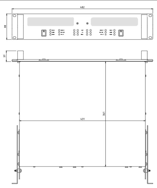
The DNA 5K4c DSP amplifier system is designed to be mounted in a standard 19" equipment rack enclosure.
