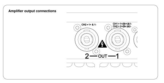
The Speakon<sup>™</sup> connector for amplifier channel 1 carries the output for amplifier channels 1 and 2. In addition this connector can also be used if the pair of amplifier channels is being operated in bridged mode.
