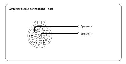
Additionally, the channel 2 output is duplicated on the Speakon<sup>TM</sup> connector for amplifier channel 1 for Bi-Amp wiring. Similarly, the channel 4 output is duplicated on the Speakon<sup>TM</sup> connector for amplifier channel 3. This can be useful for making a connection to two loudspeakers with one 4-core cable (i.e. Bi-Amp).
