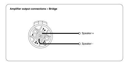
More than one speaker can be connected to each channel provided the total impedance per channel is not less than **2 ohms**. In bridged mode the minimum total impedance should not be less than **4 ohms**.
