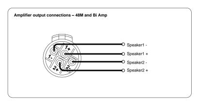
In addition, the channel 1 or channel 3 connector (all the Speakon<sup>TM</sup> connectors on the 48M model) can also be used if the pair of amplifier channels is being operated in bridged mode.
