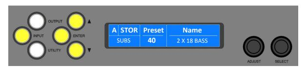
Note: Storing a Drive Module preset for a module which is not configured with consecutive outputs is not permitted.
