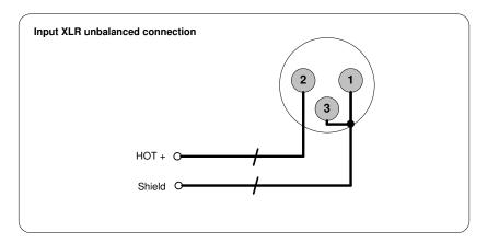
An unbalanced input may be driven by connecting pin-3 'cold' signal to the ground connection of the unbalanced destination input. The cable shield is connected to pin 1 at the source (this device), and to ground at the destination device (along with the pin 3 'cold' connection). Alternatively, if the cable is a single core plus shield, the cable shield should be terminated to both pins 1 and 3.
