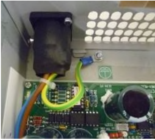
Mains inlet and earth wiring
