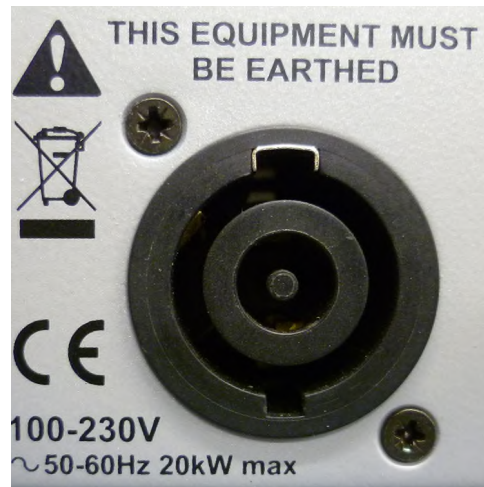
Mains input markings (rear)
