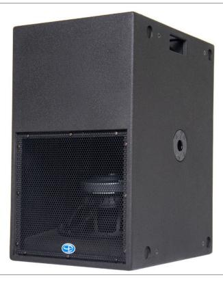
The THMini15 is a variation of the popular THMini. Unlike the original THMini, it utilizes (1) x 15" long excursion LF driver. The Danley Tapped Horn Subwoofer ™ is a patented design that allows us to build physically small subs which are very efficient, especially at the low end of their range, and are virtually linear in their passband.
