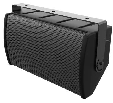
The SM100 utilizes the same patented Synergy Horn™ technology as the renowned SH Series but employs a molded horn technique to save weight. The SM100 features a 8"/1" coaxial driver mated to a wide 100 degree conical horn that maintains excellent pattern control to very low frequencies despite its compact size. Overall frequency response and fidelity are other hallmark features of the oldest full range loudspeaker in the Danley catalog.
