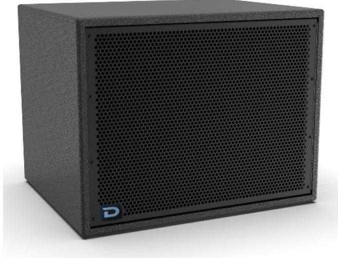
The AXS15 is a compact, high-output subwoofer system engineered around a 15-inch long-excursion low-frequency transducer housed in a front-loaded, bass-reflex enclosure. The dual-vent system is optimized to minimize turbulence and port compression under high-SPL conditions, with a tuning frequency of 35 Hz to deliver extended low-frequency performance and stable operation at elevated power levels.
